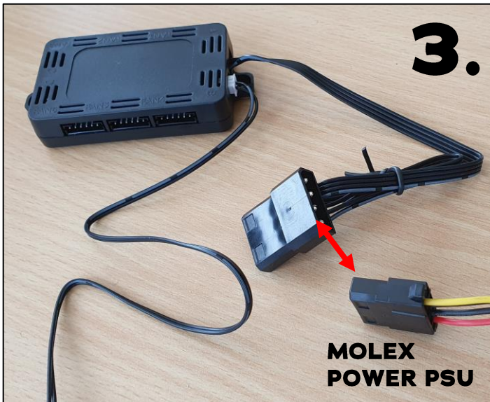
3. Connect the Molex Power from the controller to your PSU
